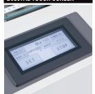
The touch screen control module comes pre-programmed with 83 cutting templates.
