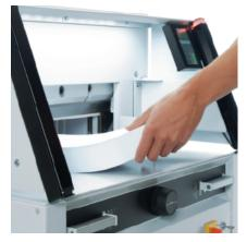
**IR SAFETY CURTAIN** The IR light beam safety curtain covers the work area to ensure the highest level of operator safety.
