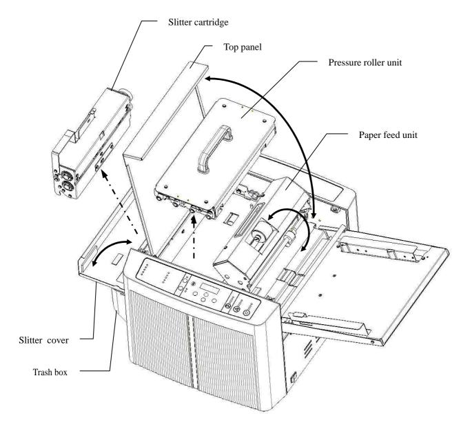
\* The main remedy for handling paper jams are explained later in this manual. Deal with it according to the location and type of error.
