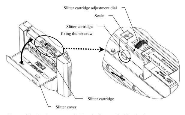
\* After completing the adjustment, securely tighten the slitter cartridge fixing thumbscrew.
